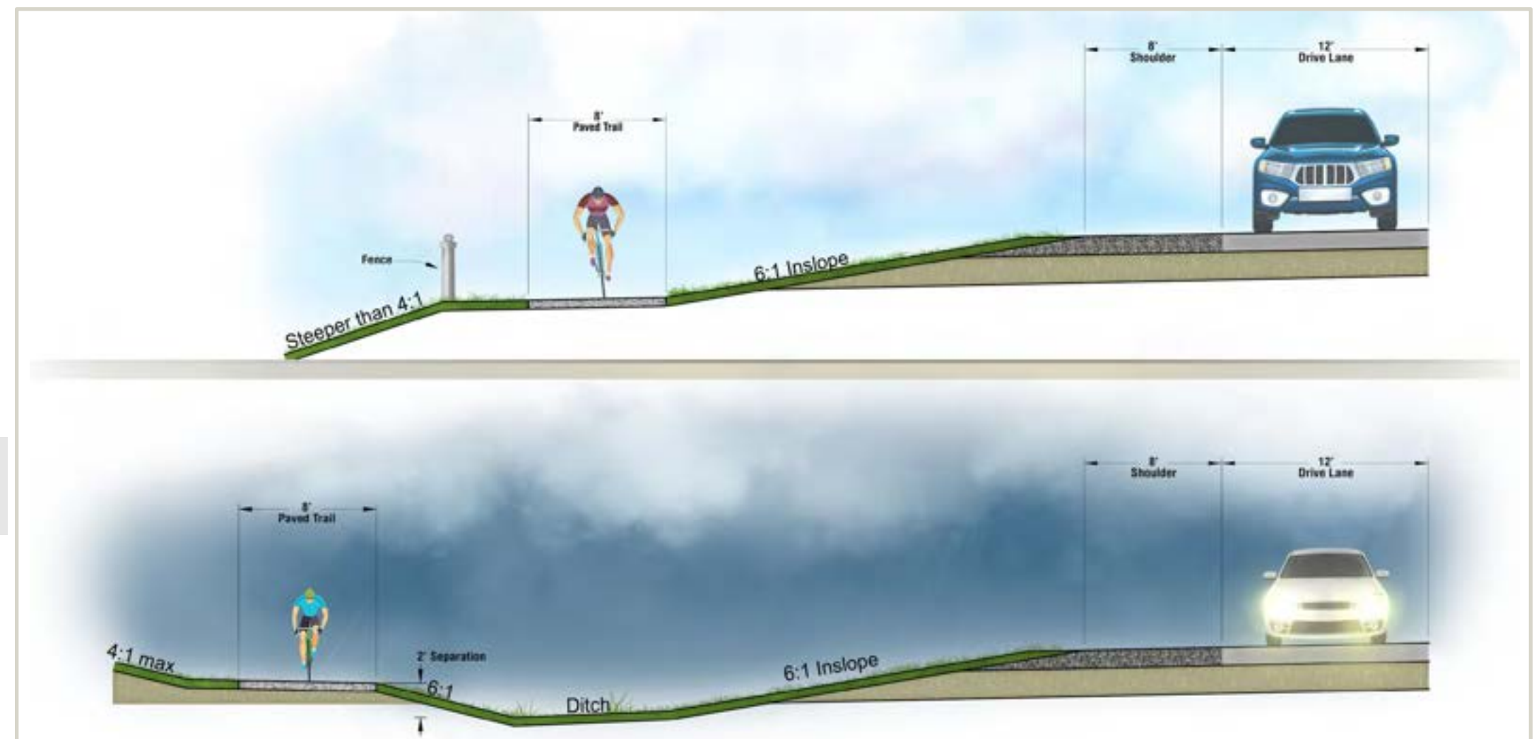
Figure 42, Trail Typical Sections
