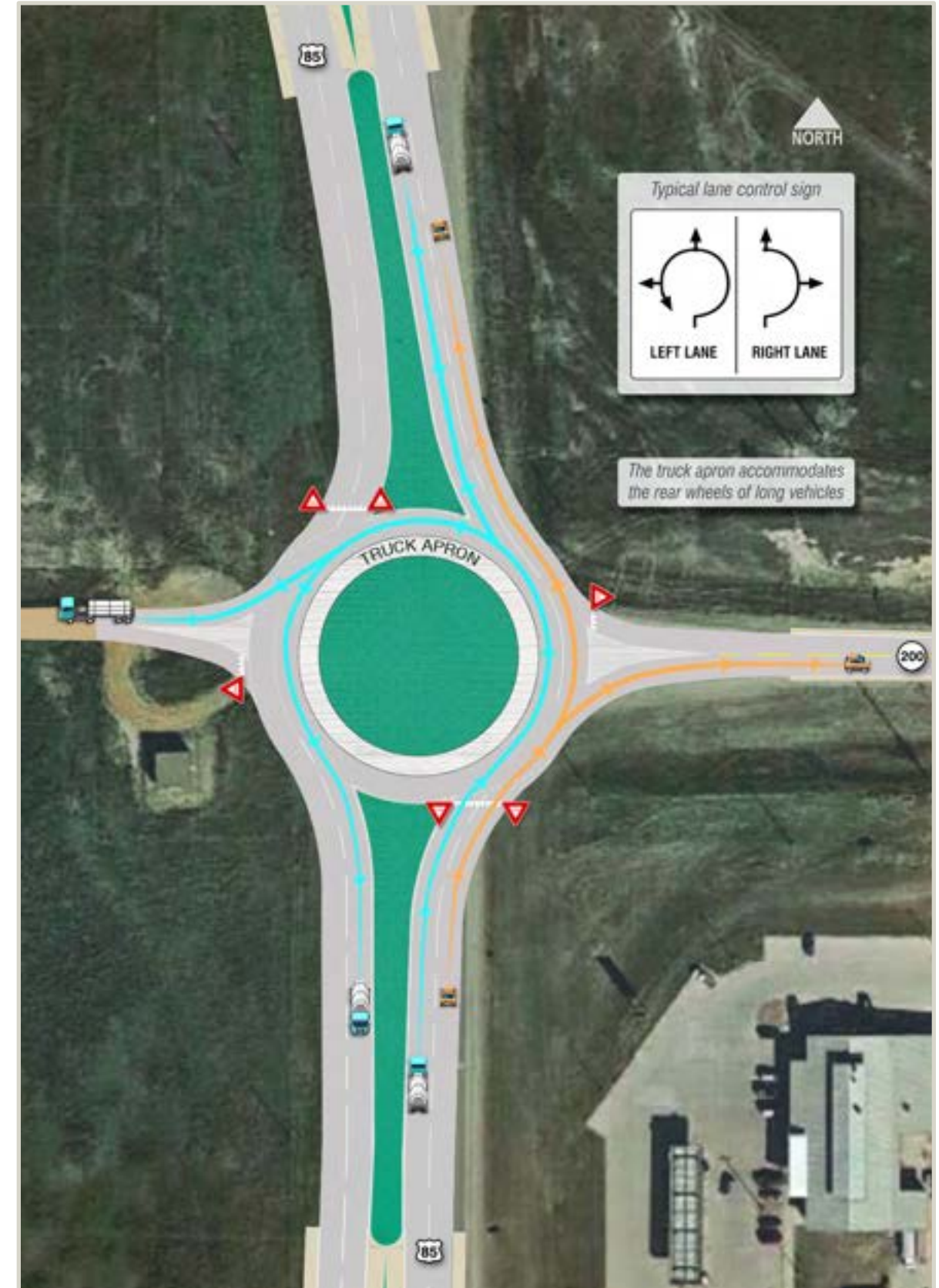
Figure 24, Multi-lane Roundabout Illustration
