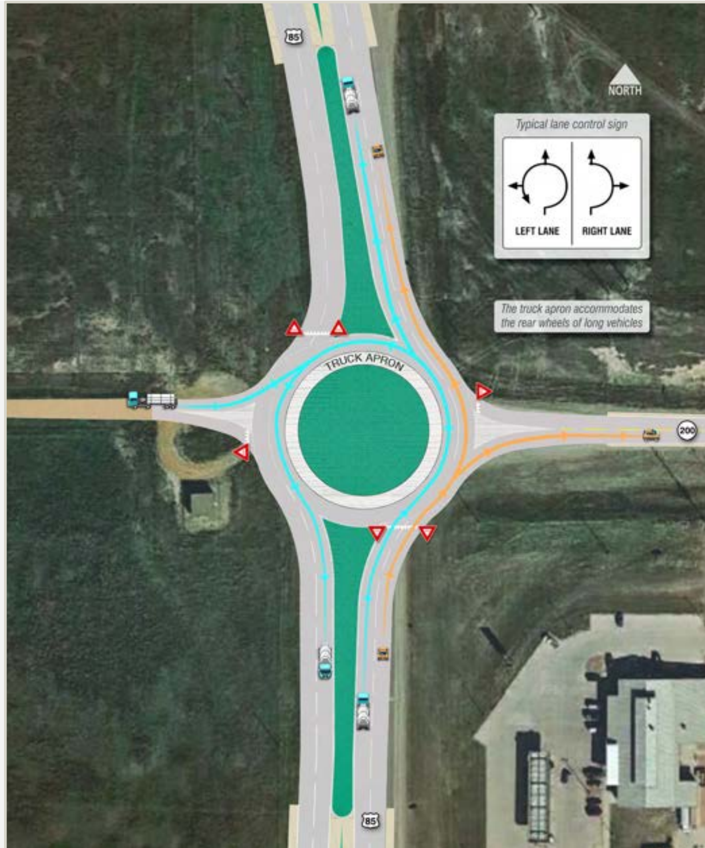
Figure ES-6, Multi-lane Roundabout Illustration
