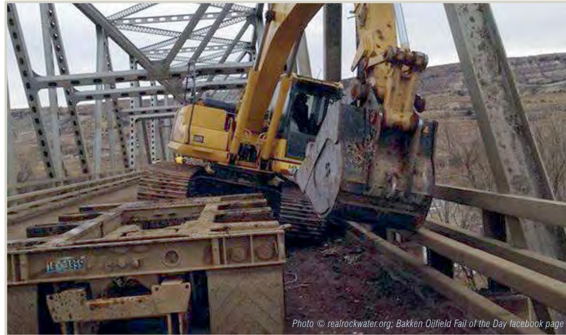
Figure 84, Load shifted off trailer after collision with Long X Bridge overhead member
